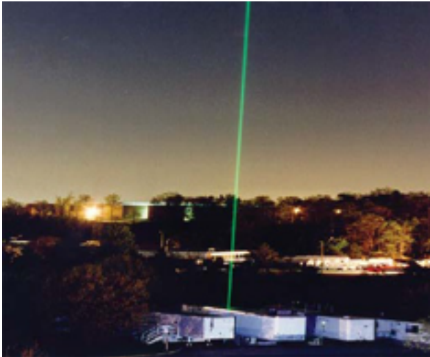
AT Lidar operating at GSFC; 532 nm beam is clearly visible.
