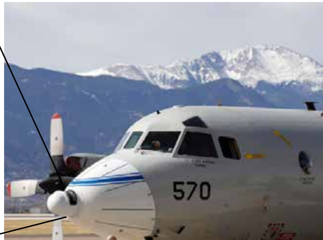
Schematic illustration of NASA's Cloud Absorption Radiometer (CAR) mounted in the nose of the Naval Research Lab (NRL P-3C) aircraft during the SnowEx field experiment based out of Colorado Springs, Colorado, USA, in 2017 (picture credit: The Associated Press).
