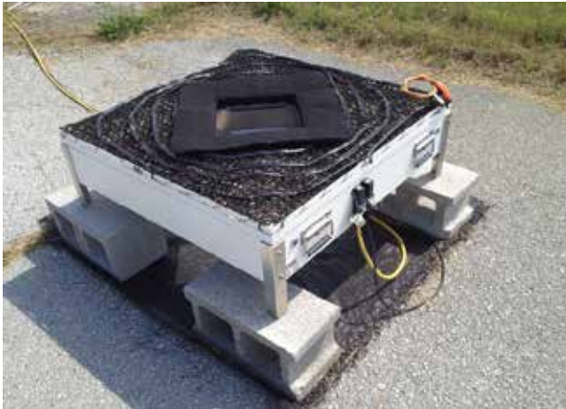
A 2DVD as commonly deployed. The unit is elevated on cinder blocks to help mitigate splashing of rain drops by the ground. The drops fall through the center of the instrument and are simultaneously imaged by two orthogonal cameras.
