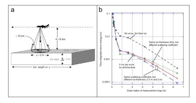
Concept of new lidar measurements of snow and sea ice thickness
