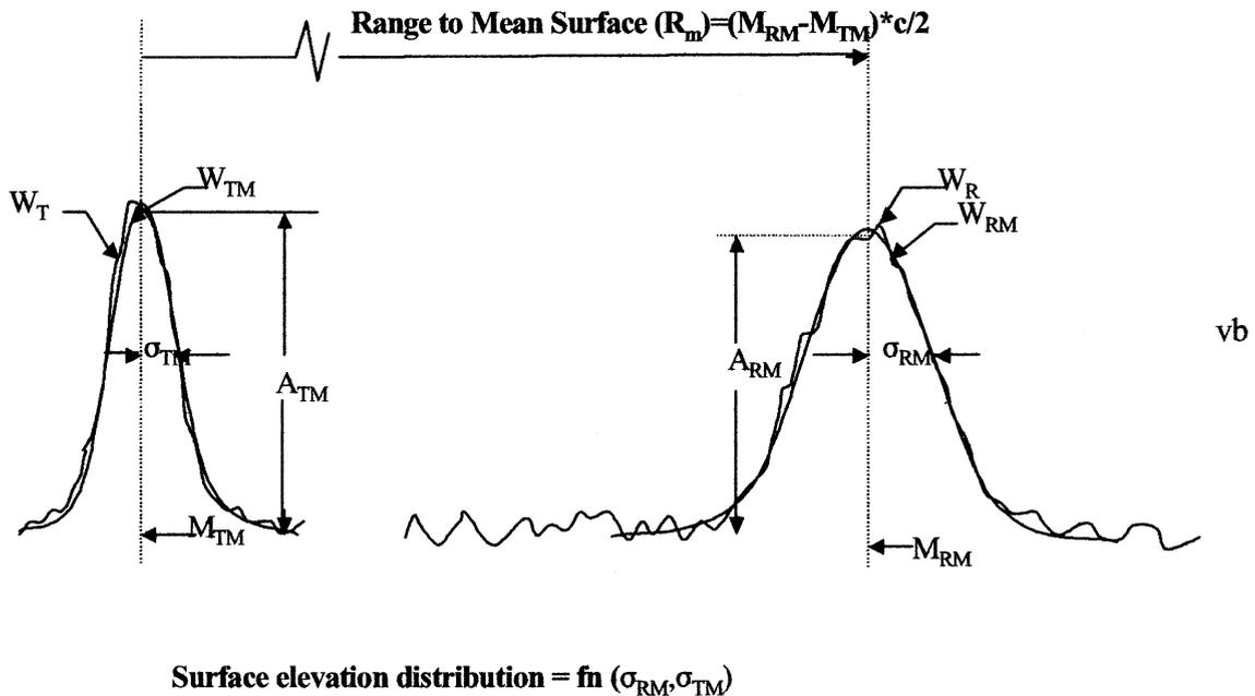
Fig. 7.1. Calculation of range and elevation distribution from typical transmitted and received GLAS pulses. *W* indicates the pulse or modeled waveform, *T* indicates the transmitted pulse, *R* indicates the received pulse, subscript *M* refers to the Gaussian model fitted to the waveform, *M* indicates the waveform mid-point, and  $\sigma$  indicates the standard deviation of the waveform.
