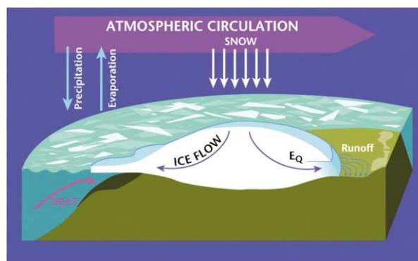
Fig. 1.2. Snow accumulation on the polar ice sheets is approximately balanced by ice flow toward the margins where the ice below the equilibrium line (EQ) melts or calves into icebergs. Changes in the annual water exchange of about 8 mm of global sea level can be caused by changes in the atmospheric/ocean temperatures or circulations or by internal changes in the ice dynamics. A 1 m change in the average ice-sheet thickness of 2360 m would cause a global sea level change of about 4 cm.
